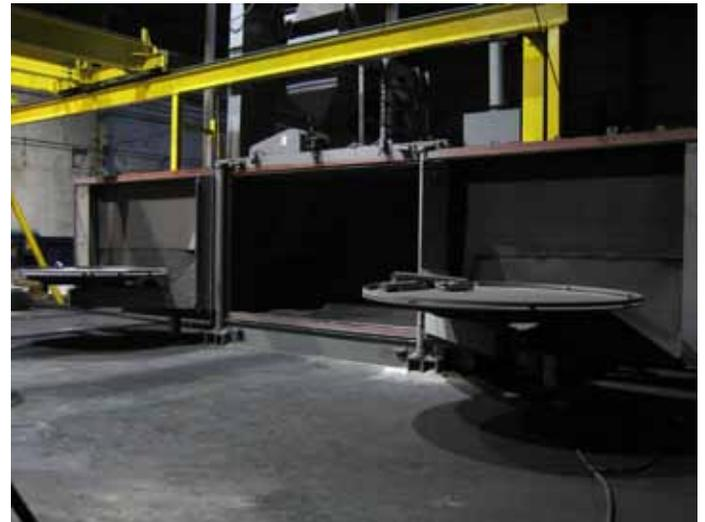
Our double door table blast allows quick and efficient processing of castings.
