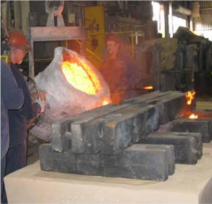
Quaker City Castings produces sand molds using the AlphaSet no-bake molding system, giving us great dimensional flexibility as well as the ability to pour castings up to several thousand pounds. We can produce **steel castings up to 5,000 lbs.** (2,722 kg) and **iron castings up to 12,000 lbs.** (5,443 kg). All melting is accomplished using a combination of channel induction furnaces and coreless induction furnaces.
