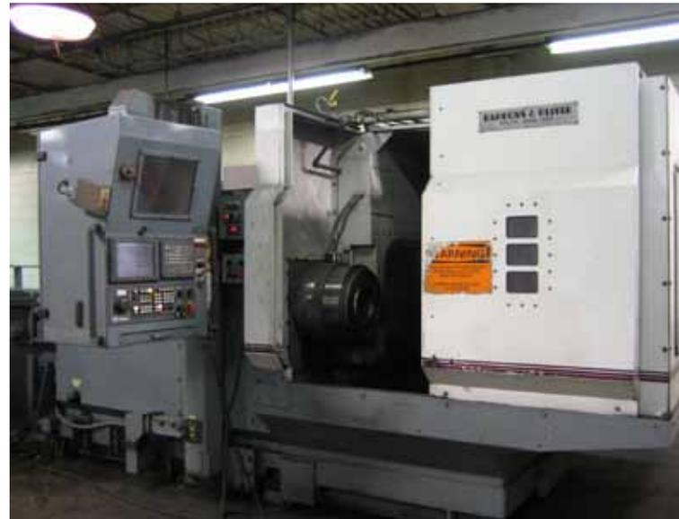
Our big bore lathes can finish-machine centrifugal castings up to 8" diameter.
