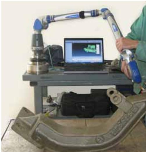
Dimensional accuracy measured with the FARO Edge.
